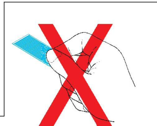
1. Separate the etched components from their frames on the protective paper. Removal from the paper is done only after separation of the parts from the frames.
